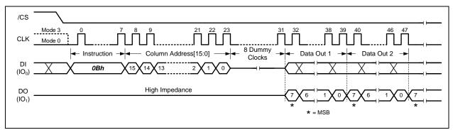
Figure 8-21 Fast Read Instruction (Buffer Read Mode, BUF=1)
