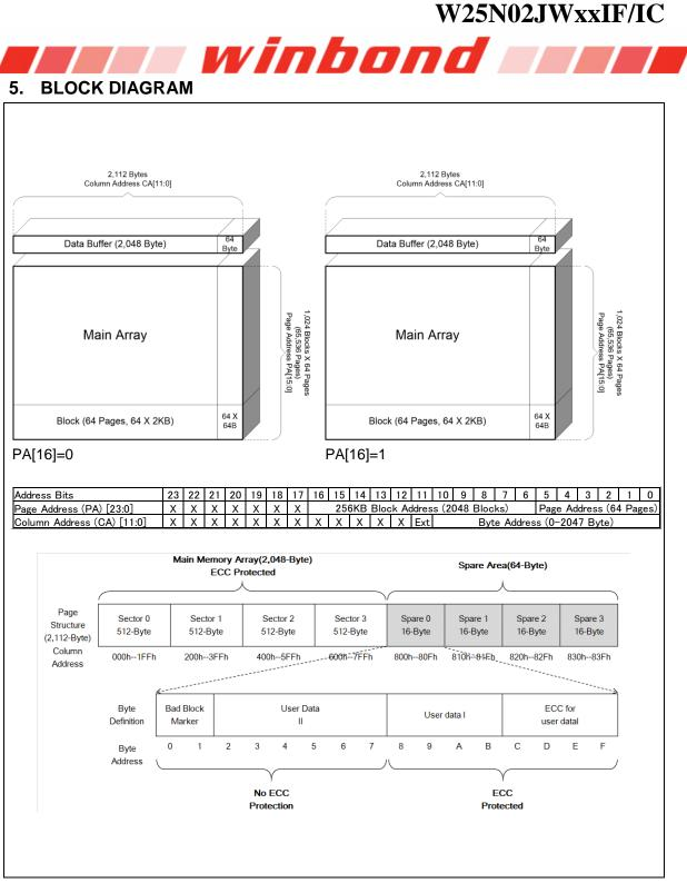
Figure 5-1 W25N02JW Flash Memory Architecture and Addressing
