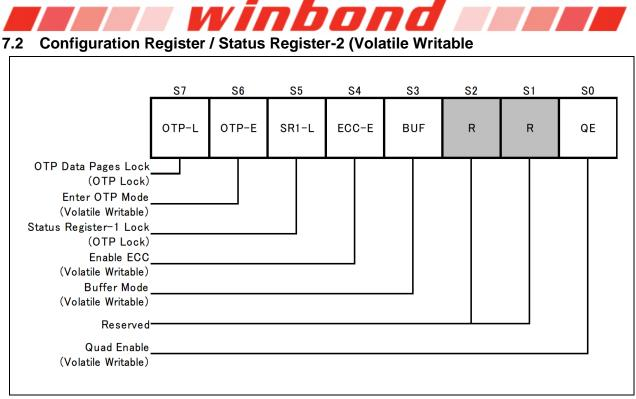
Figure 7-2 Configuration Register / Status Register-2 (Address Bxh)
