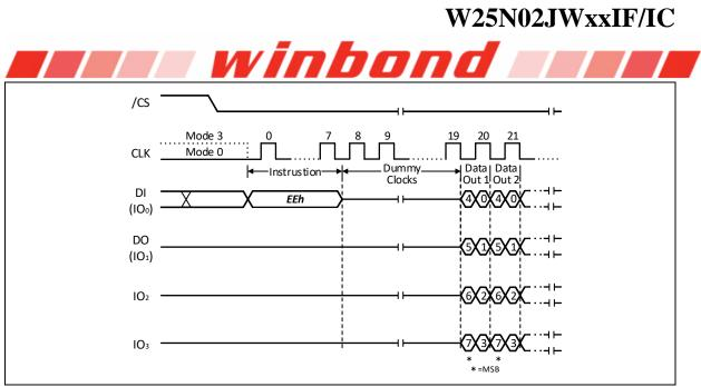
Figure 8-56 DTR Fast Read Quad I/O Instruction (Continuous Read Mode, BUF=0)
