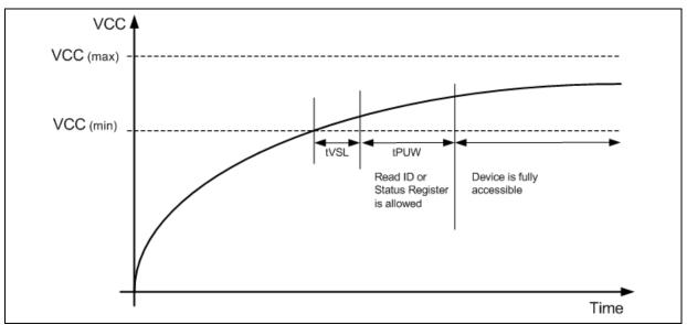
Figure 9-1 Power-up Timing and Voltage Levels
