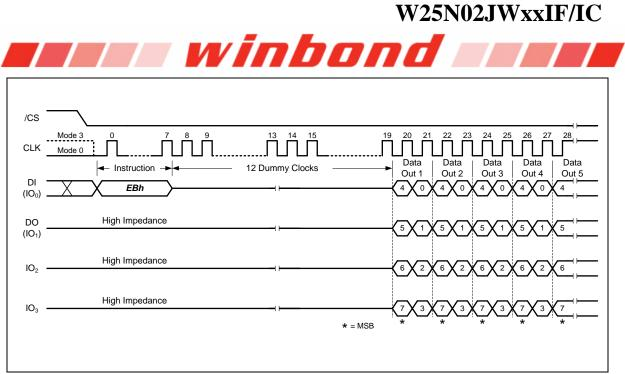
Figure 8-38 Fast Read Quad I/O Instruction (Continuous Read Mode, BUF=0)
