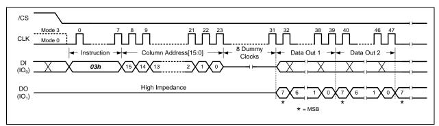
Figure 8-19 Read Data Instruction (Buffer Read Mode, BUF=1)
