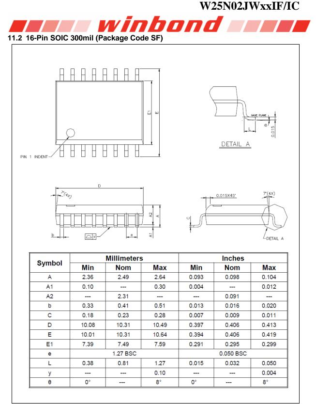
Figure 11-2 16-Pin SOIC 300mil (Package Code SF)
