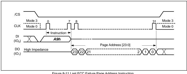
Figure 8-11 Last ECC Failure Page Address Instruction
