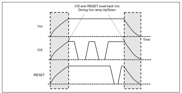
Figure 9-2 Power-up, Power-Down Requirement
