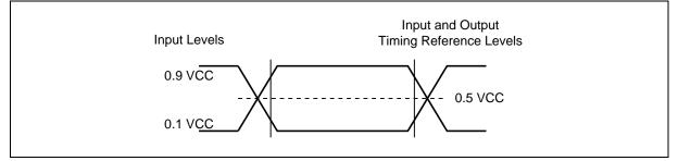
Figure 9-3 AC Measurement I/O Waveform
