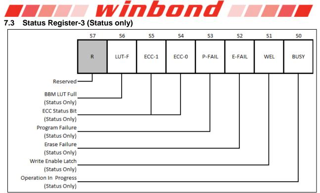
Figure 7-3 Status Register-3 (Address Cxh)
