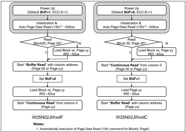
Figure 6-1 W25N02JW Flash Memory Operation Diagram
