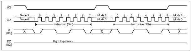
Figure 8-2 Device Reset Instruction (66h+99h)
