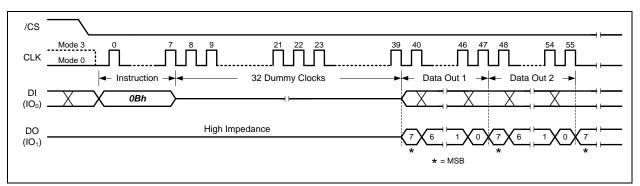
Figure 8-22 Fast Read Instruction (Continuous Read Mode, BUF=0)
