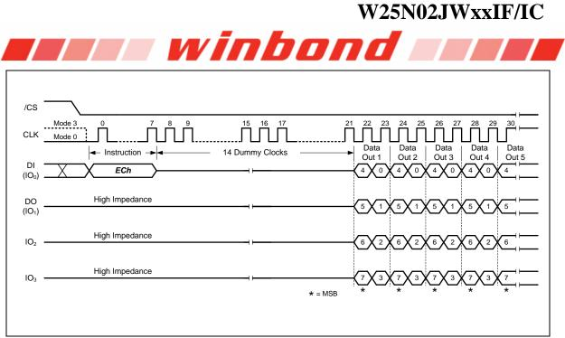
Figure 8-40 Fast Read Quad I/O with 4-Byte Address Instruction (Continuous Read Mode, BUF=0)
