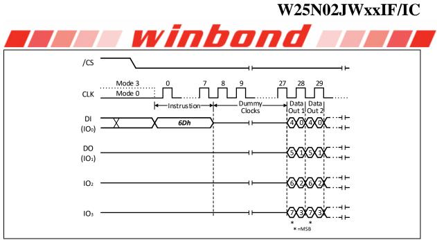
Figure 8-48 DTR Fast Read Quad Output Instruction (Continuous Read Mode, BUF=0)
